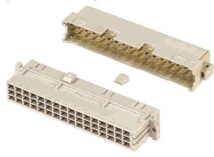
To avoid cross-plugging of adjacent connectors a coding system is required. Insert the code key 09 06 001 9919 into one of the keyways of the female connector as shown in the drawing. Break out the corresponding area of the male shroud. Connectors coded this way can only be applied in a minimum rack spacing of 20.32 mm.
